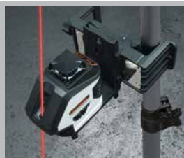
Additional plumb laser at top and bottom
